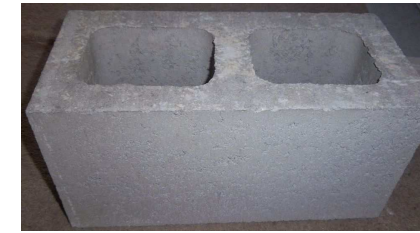
Low cost concrete blocks from reclaimed aggregates
