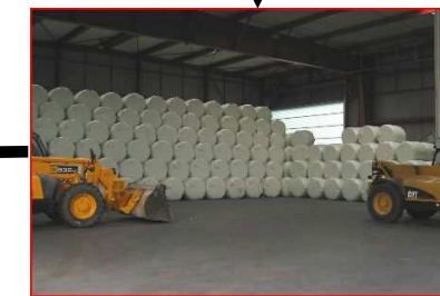
MSW Fiber is White Baled in 3 tons packs for distribution directly to PowerCan® 200 station hoppers
