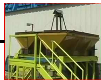
The CHP Hopper Units screw feeds "White Baled" MSW fiber feedstock bales 24hrs per day
